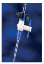
Borosilicate glass, single bore, interchangeable stopcocks, blue ceramic 0.10mL graduations
